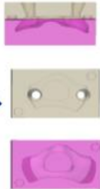
Create mold of insert and inject with silicone
